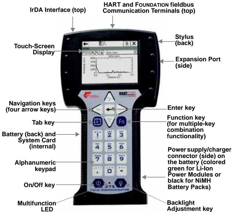
Figure 2-3. 375 Field Communicator diagram
